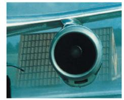
AHI roofs withstand the toughest wind testing.
