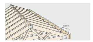
Using the measuring rod (pre-notched at 368 mm for shingles) hook it over the nail so that it lies up the rafter. Tack a batten nail in each slot as markers for the battens. (Fig 2.2.3).
