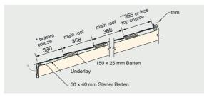
\* Variable depending on the type of rainwater collection system used. \*\* Dimensions will vary depending on rafter length.
