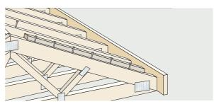
Two common methods of installation are with an intermediate (centre) batten (Fig 2.1.1) or using a single wide batten (Fig 2.1.2).
