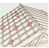
(Fig 2.2.4) and cut the battens to length so that they butt together on top of a rafter. Hold the batten firmly against the marking nail and nail through each batten into the rafter. Once installed, pull out the marking nail and use it fix the next batten.
