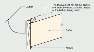
Where a rainwater collection system is not used and the shingle overhangs the fascia, secure a  $50 \times 25$  mm dressed batten to the front edge before the shingles are laid. (Fig 1.4.2).
