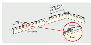
\* Variable depending on the type of rainwater collection system used. \*\* Dimensions will vary depending on rafter length.
