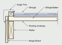
Finish junctions of barge and ridge, scribing accessories to fit - seal the joint and rivet together. (Figs 4.1.3 and 4.1.4).
