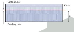
Place the full shingle in the long tile bending attachment which can be bolted to the bender. Line up the marks showing the bend line and bend the shingle upwards. Shingles can be bent in either the bender or, depending on the length, with the long tile bending attachment. Finally, cut along the marked cutting line using the guillotine or hand shears.
