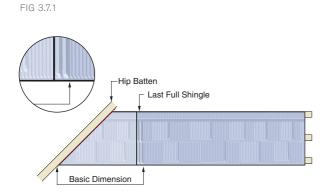
(iii) Measure and mark on the shingle with chalk or similar. The measurement is done from the edge of the lap on the shingle adding the basic measurement dimension taken from the roof, the angle is marked using the bevel. This is the bend line for the hip shingle. Add 40 mm to the bend line measurement to create the cut line (as shown in Fig 3.7.2).
