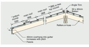
Variable depending on the type of rainwater collection system used. \*\* Dimensions will vary depending on rafter length.
