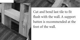
Then add flashing, or if flashing is already there, slide tile up under flashing and secure.
